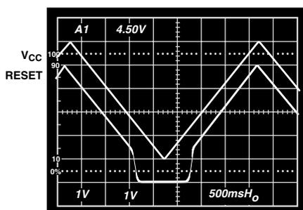
Figure 9. ADM707/ADM708  $\overline{\text{RESET}}$  Output Voltage vs. Supply Voltage
