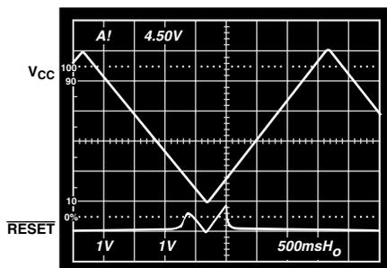
Figure 8.  $\overline{\text{RESET}}$  Output Voltage vs. Supply Voltage
