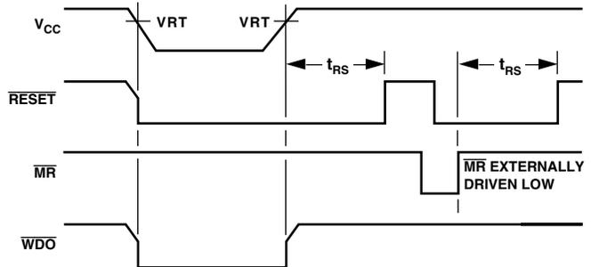
Figure 3.  $\overline{\text{RESET}}$ ,  $\overline{\text{MR}}$ , and  $\overline{\text{WDO}}$  Timing
