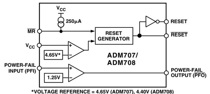
Two supply-voltage monitor levels are available. The ADM705/ADM707 generate a reset when the supply voltage falls below 4.65 V, while the ADM706/ADM708 require that the supply fall below 4.40 V before a reset is issued.
