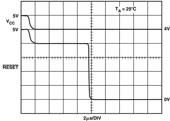
Figure 14. ADM705/ADM707  $\overline{RESET}$  Response Time
