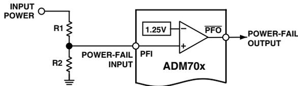
Figure 5. Power-Fail Comparator
