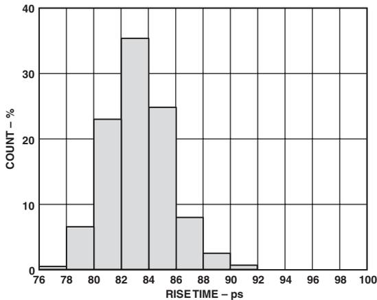
Figure 4. Rise Time Distribution Under Worst-Case Operating Conditions
