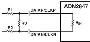
NOTE THAT  $R_{IN} = 100\Omega$  = THE DIFFERENTIAL INPUT IMPEDANCE OF THE ADN2847
