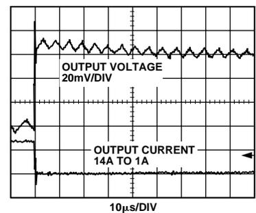
Figure 9. Transient Response, 14 A-1A of Figure 2 Circuit
