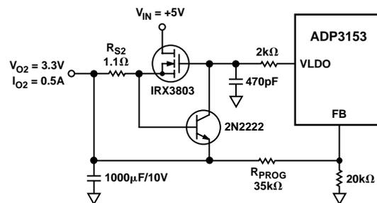
Figure 14. Linear Regulator with Overcurrent Protection
