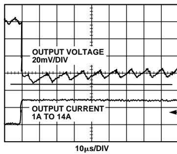
Figure 10. Transient Response, 1A-14 A of Figure 2 Circuit
