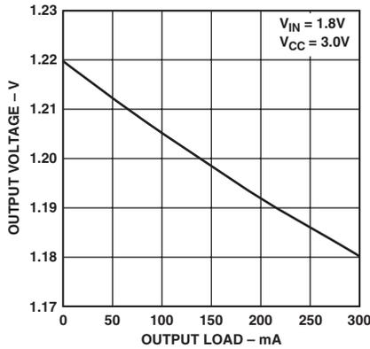
TPC 2. Output Voltage vs. Load Current
