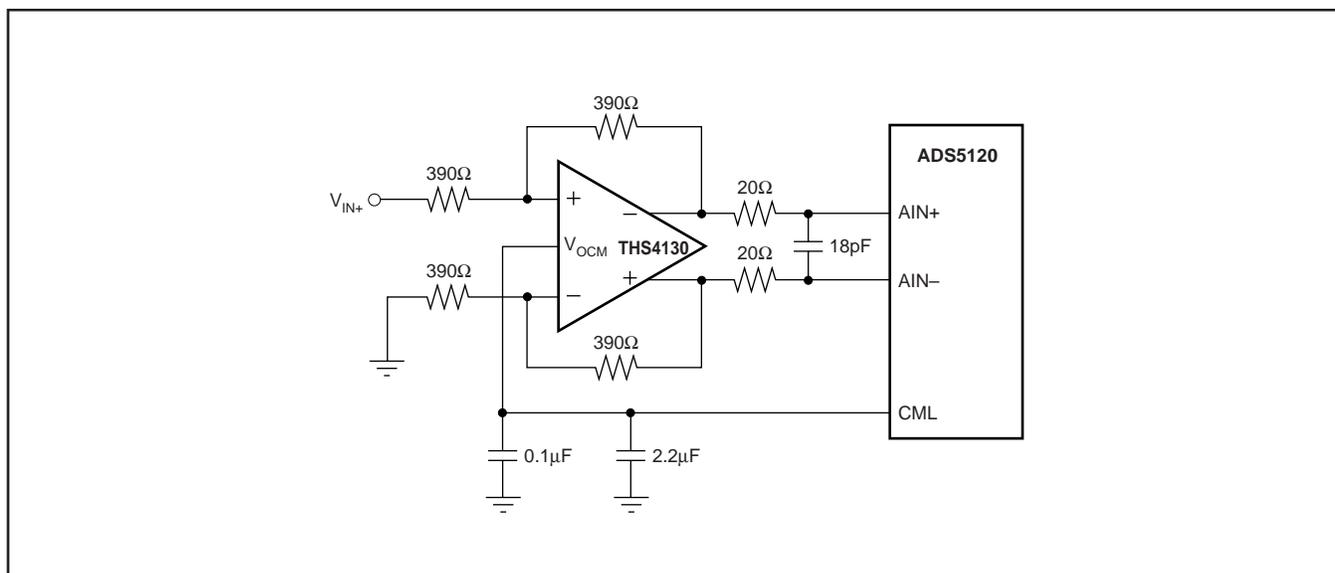
FIGURE 4. DC-Coupled Interface Using Differential I/O Amplifier THS4130.
