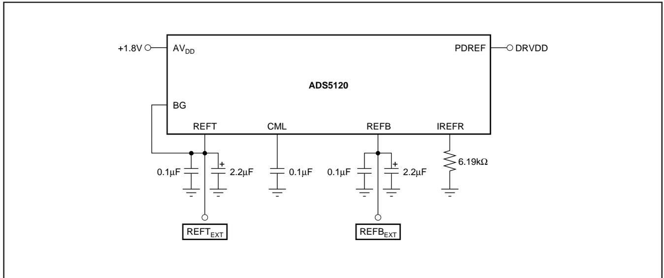
FIGURE 6. External Reference; Recommended Configuration and Bypassing.
