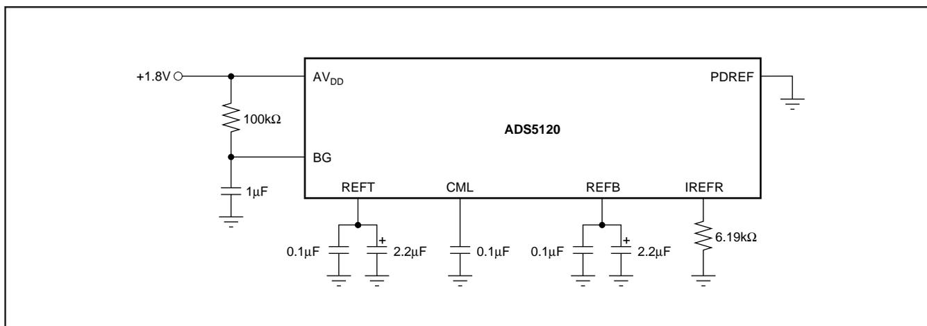
FIGURE 5. Internal Reference; Recommended Configuration and Bypassing.
