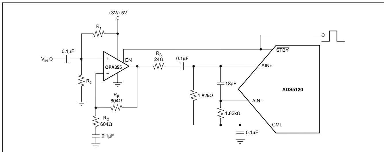
FIGURE 3. Single-Ended, AC-Coupled Driver Configuration for Single Supply.
