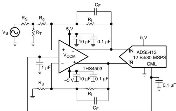
Figure 32. Using the THS4503 With the ADS5413
