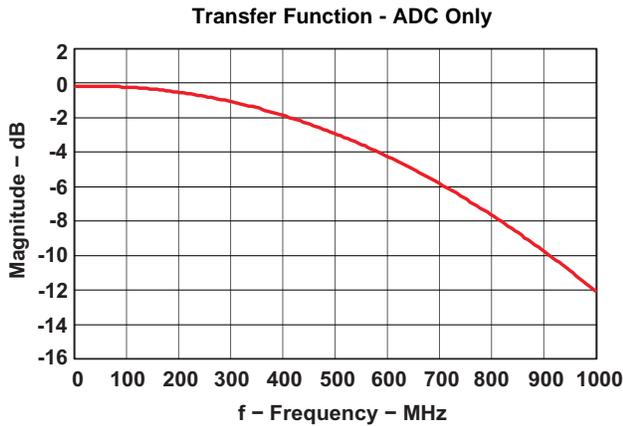
Figure 42. Analog Input Bandwidth (Data From Actual Silicon)
