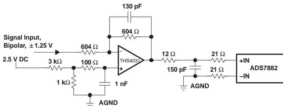
Figure 35. Typical Analog Input Circuit for Bipolar Signal
