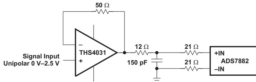
Figure 36. Typical Application Input Circuit for Unipolar Signal
