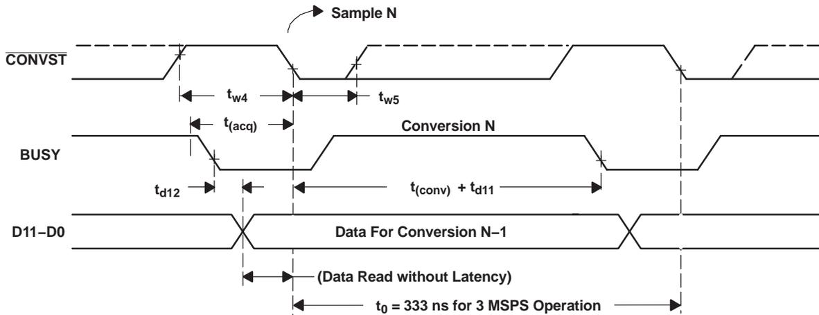
Figure 7. Back-To-Back Operation With  $\overline{CS}$  and  $\overline{RD}$  Low
