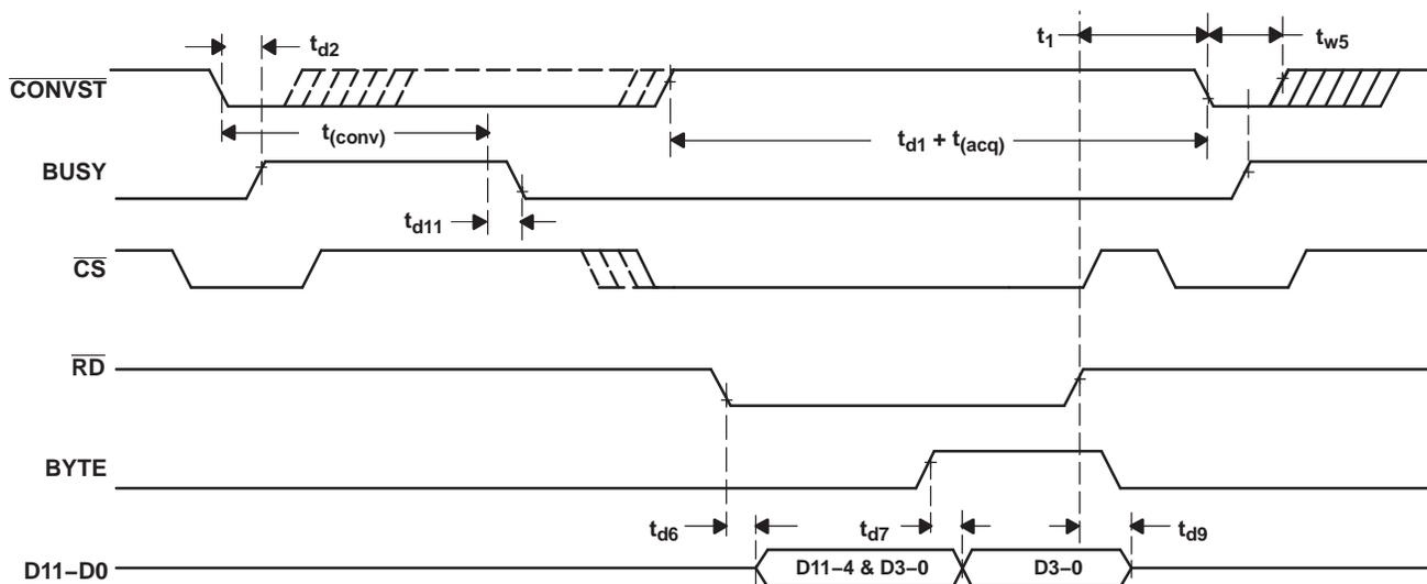
Figure 5. Read Control via  $\overline{CS}$  and  $\overline{RD}$
