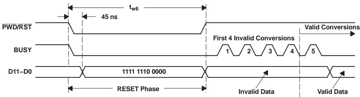
**Figure 12. Device Reset**
