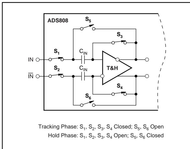
FIGURE 1. Simplified Circuit of Input Track-and-Hold Amplifier.
