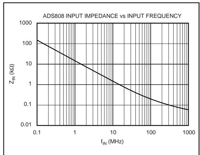
FIGURE 2. Differential Input Impedance versus Input Frequency.
