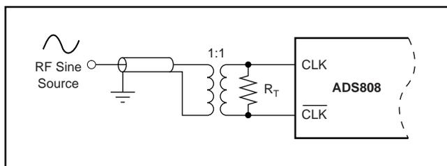
FIGURE 12. Applying a Sinusoidal Clock to the ADS808.
