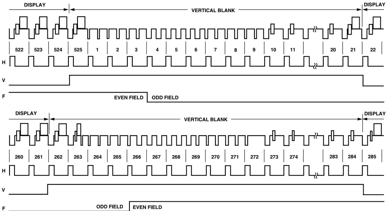
Figure 8. Timing Mode 0 (NTSC Master Mode)
