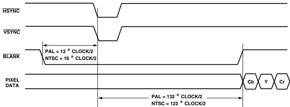
Figure 16. Timing Mode 2 Even-to-Odd Field Transition Master/Slave
