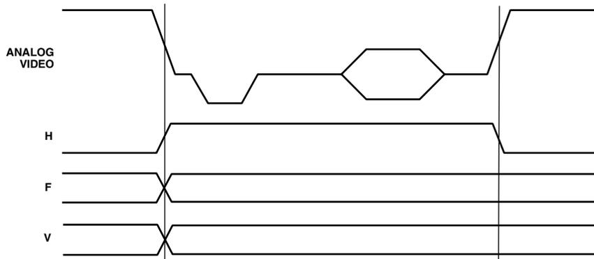
Figure 10. Timing Mode 0 Data Transitions (Master Mode)
