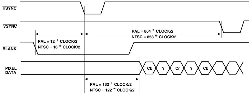
Figure 17. Timing Mode 2 Odd-to-Even Field Transition Master/Slave
