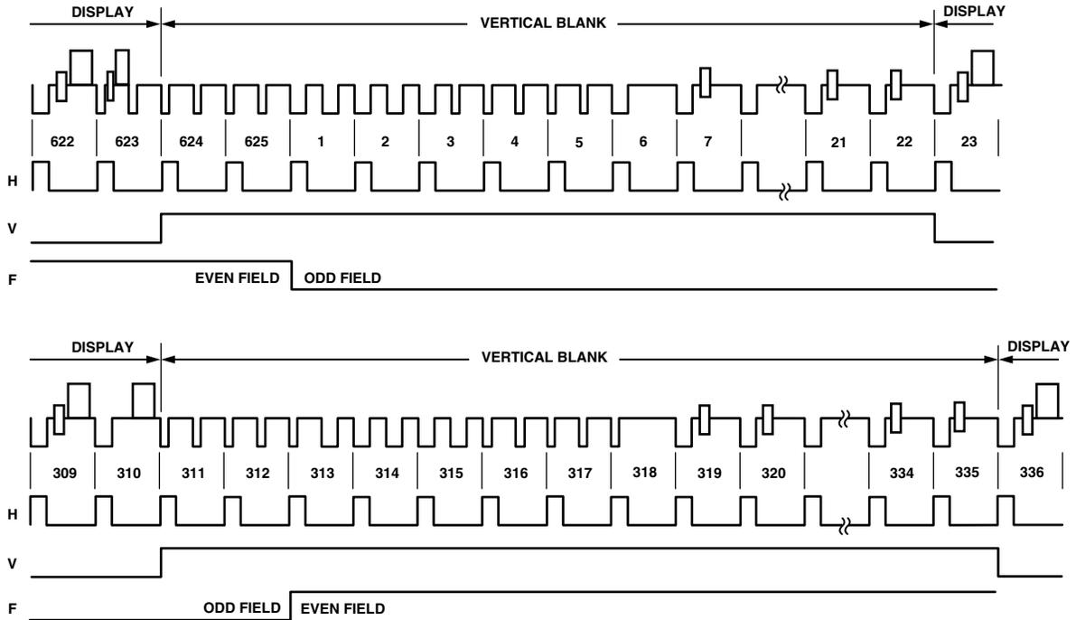
Figure 9. Timing Mode 0 (PAL Master Mode)
