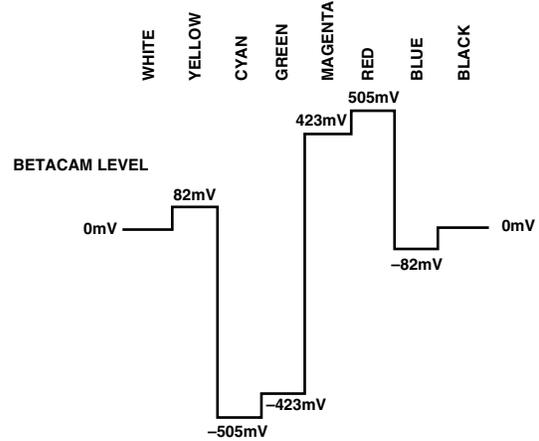
Figure 53. NTSC 100% Color Bars No Pedestal V Levels
