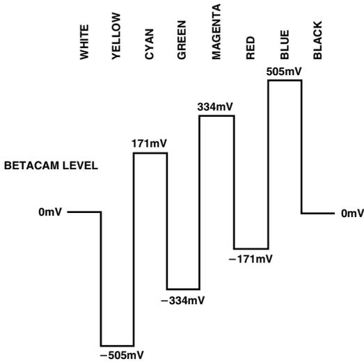
Figure 50. NTSC 100% Color Bars No Pedestal U Levels
