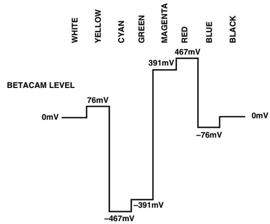
Figure 54. NTSC 100% Color Bars with Pedestal V Levels
