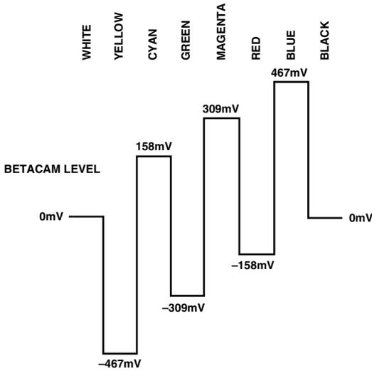
Figure 51. NTSC 100% Color Bars with Pedestal U Levels
