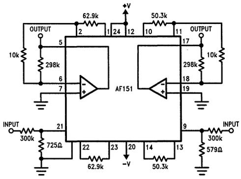
FIGURE 8. Dual Band Pass Filter
