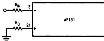
FIGURE 6. Connection for Any Q, Inverting
