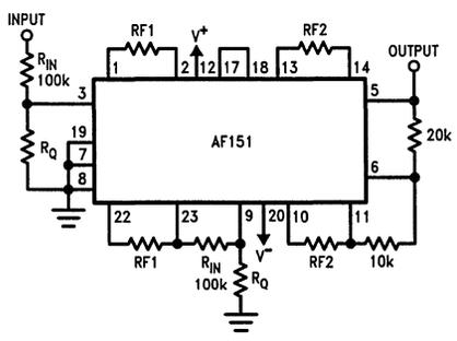
FIGURE 9. Telephone Multifrequency (MF) Band Pass Filter
