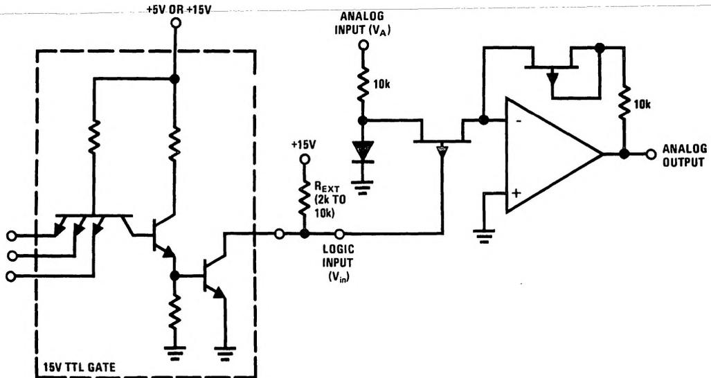
FIGURE 5. Interfacing with +15V Open Collector TTL
