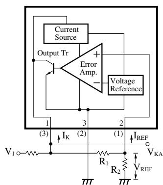
$$V_{KA} = V_{REF} \left(1 + \frac{R_1}{R_2}\right) + I_{REF} \cdot R_1$$
