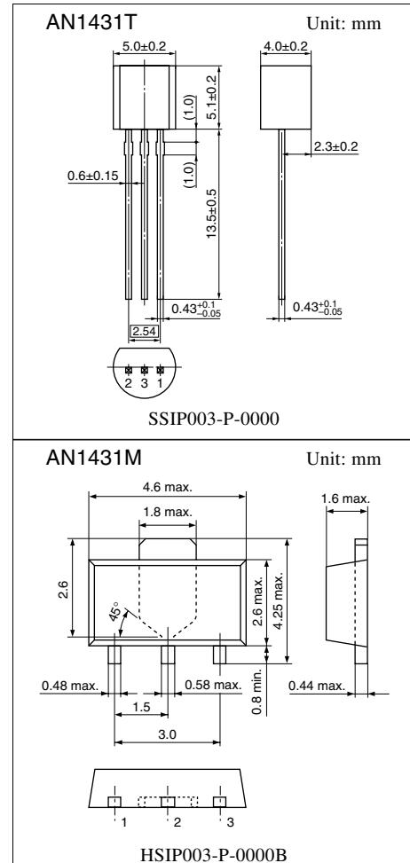
Note) The number in ( ) shows the pin number for the AN1431M.
