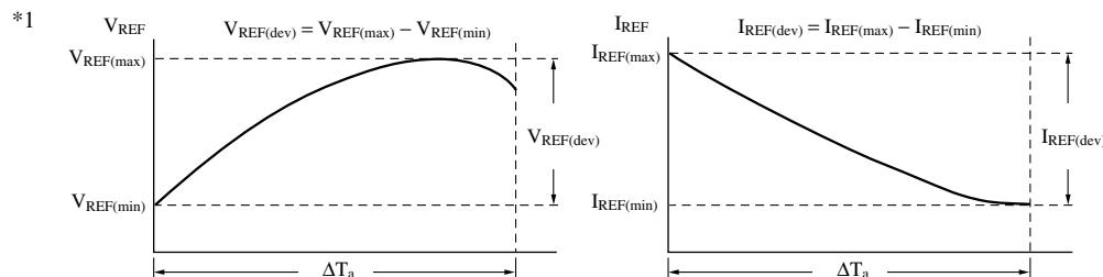
The temperature coefficient  $aV_{REF}$  for the reference input voltage is equivalently given by the following expression.
