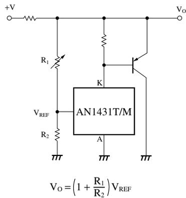
5. Adjustable output regulator combined with 3-pin regulator
