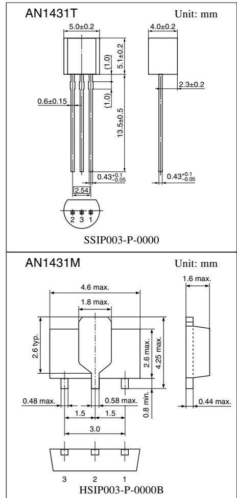
Note) The packages (SSIP003-P-0000 and HSIP003-P-0000B) of this product will be changed to lead-free type (SSIP003-P-0000S and HSIP003-P-0000Q). See the new package dimensions section later of this datasheet.
