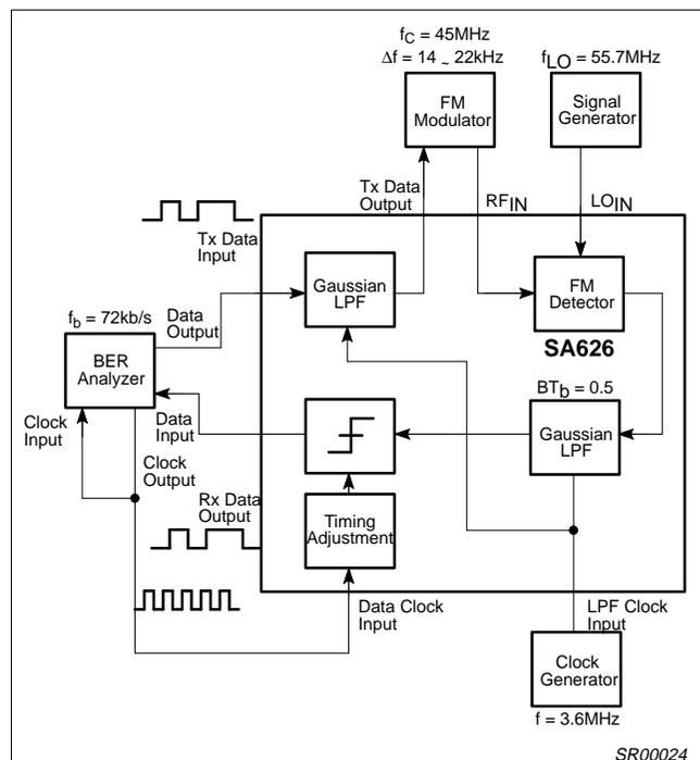
Figure 7. Measurement Set-Up with the GMSK/GFSK Board
