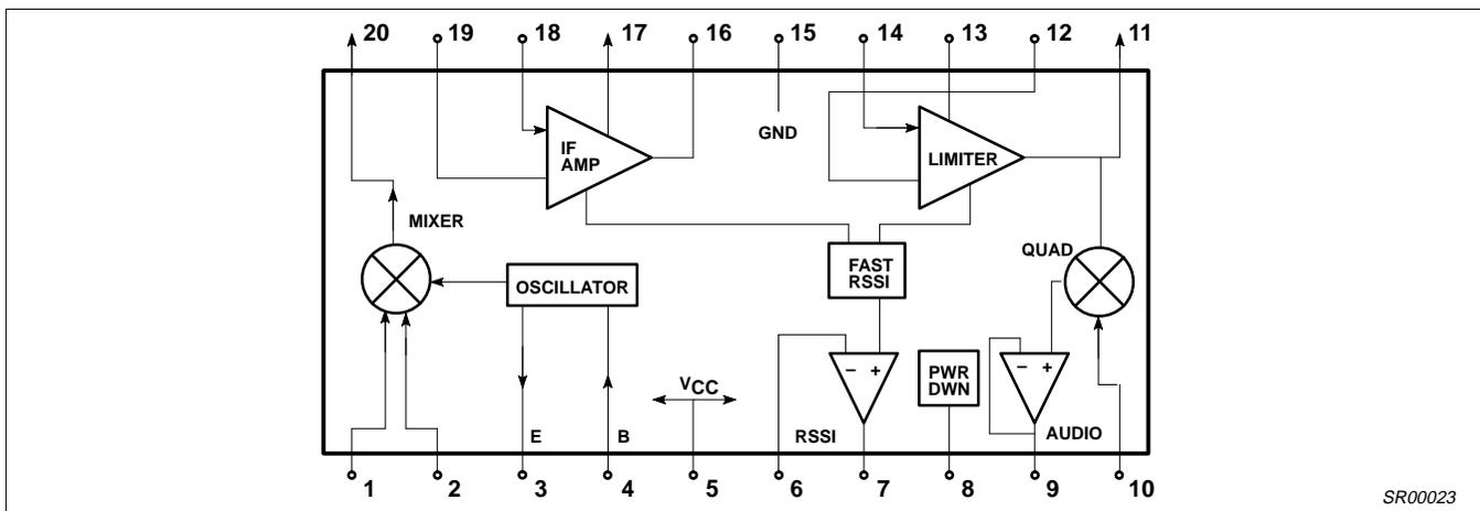
Figure 6. Block Diagram of the FM/IF System SA626
