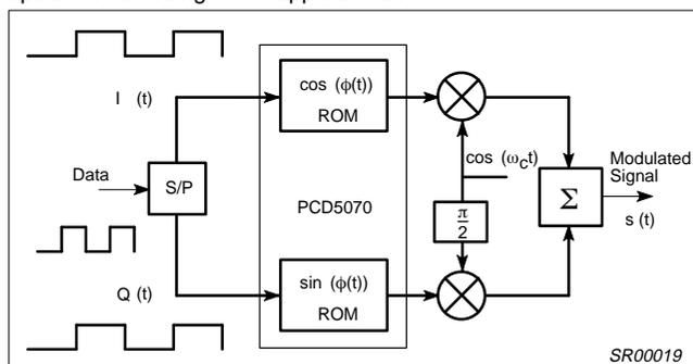
**Figure 2. I/Q Implemented GMSK Modulator**
