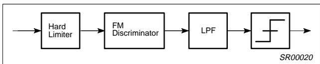
**Figure 3. Limit/Frequency Discriminator GMSK/GFSK Demodulator**
