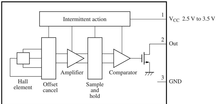
Note) The magnetism detection time should be longer than one intermittent action cycle (On = 200 μs and Off = 51 ms).
