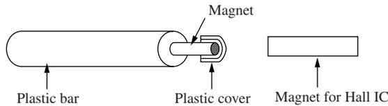
A magnet, which is used in pair with a Hall IC, can be mounted to a product incorporating a built-in Hall IC (e.g., a cellular phone) smoothly and correctly with a simple tool. The polarity of the magnet (hereafter referred to as Hall IC magnet) will be automatically discriminated.
