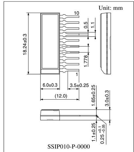
Note) The package of this product will be changed to lead-free type (SSIP010-P-0000A). See the new package dimensions section later of this datasheet.
