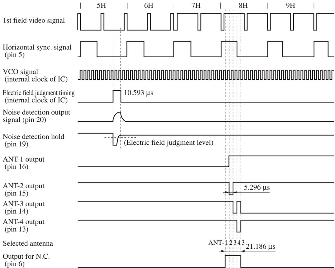
(In the above timing chart, the 1st field video signal is not an internal signal but an input signal, and some signals which do not outputted to pins, as VCO signal, are included.)
