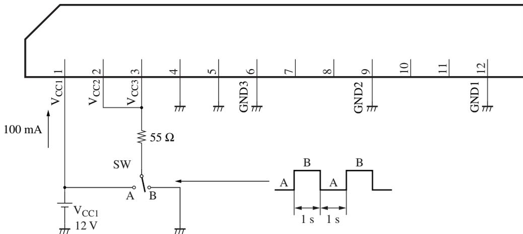
3. The change in output voltage by the V<sub>CC2</sub> and V<sub>CC3</sub> voltage change
