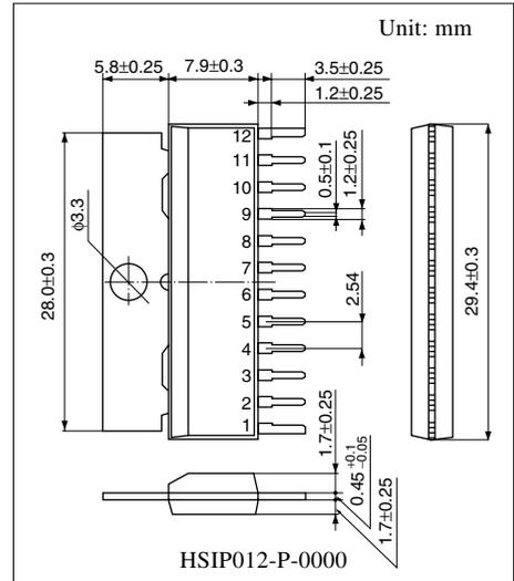
Note) The package of this product will be changed to lead-free type (HSIP012-P-0000D). See the new package dimensions section later of this datasheet.
