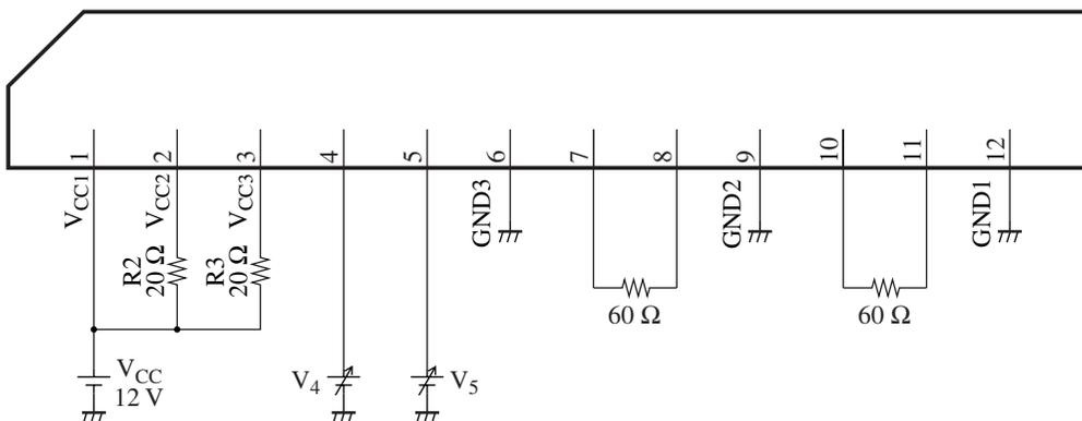
If pin 3 (V<sub>CC3</sub>) becomes a voltage of 8 V or less by making resistance value of R3 larger, the upper limit of output voltage for pin 7 and pin 8 is restricted and then the output becomes as shown in figure 1.
