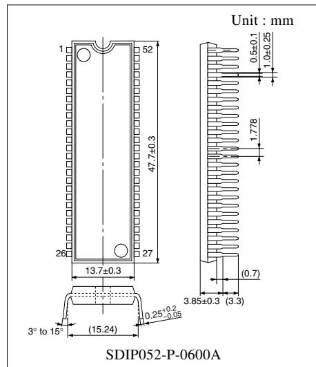
Note) The package of this product will be changed to lead-free type (SDIP052-P-0600F). See the new package dimensions section later of this datasheet.
