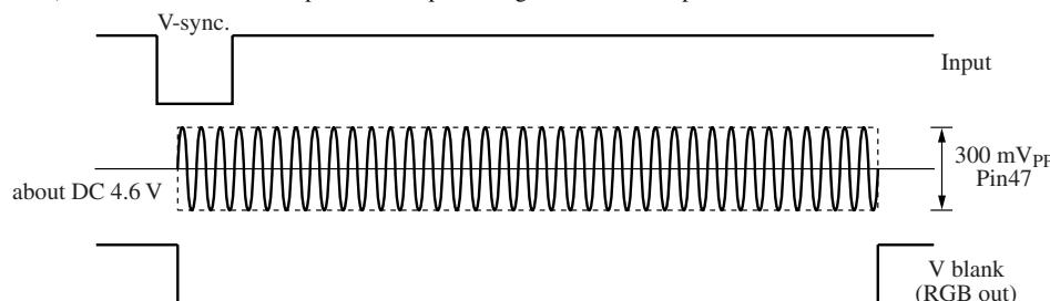
Note) \*2 : Eventhough the MICOM switches the VCO between 4.43MHz and 3.58MHz, only the 4.43 MHz CW will be outputed at periodic intervals as shown below.
