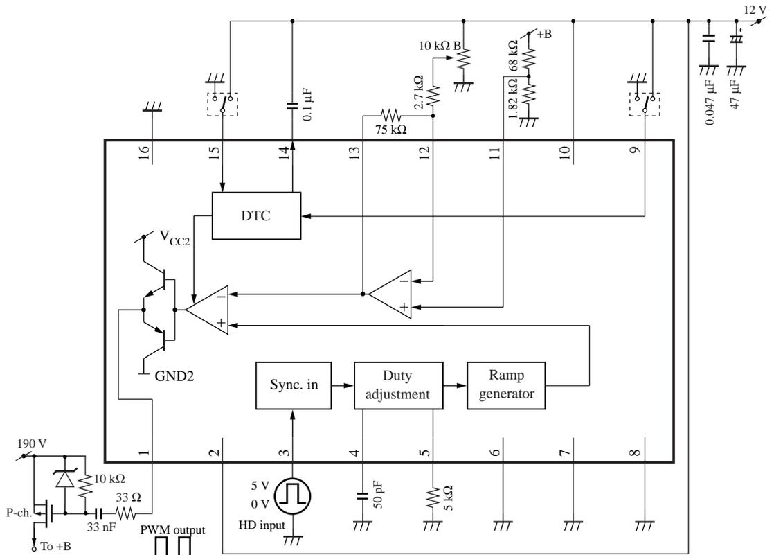
Note) When both of the pin 4 and the pin 5 are open, minimum pulse width of PWM output is 2.0 μs.
