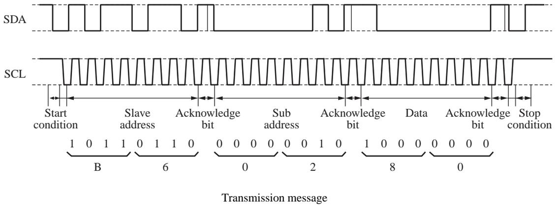
As transfer messages, SCL and SDA are transferred synchronously and serially. SCL is a constant clock frequency and SDA is address data for controlling a receiving side and is sent in parallel by synchronizing with SCL. Data are in principle sent by 8-bit 3-octet (byte) and there exists an acknowledge bit per octet. The frame structure is mentioned below:
