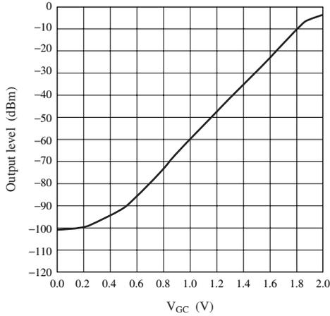
Output level — GC temperature characteristics
