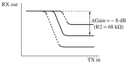
Figure 1. Variable width of attenuation
