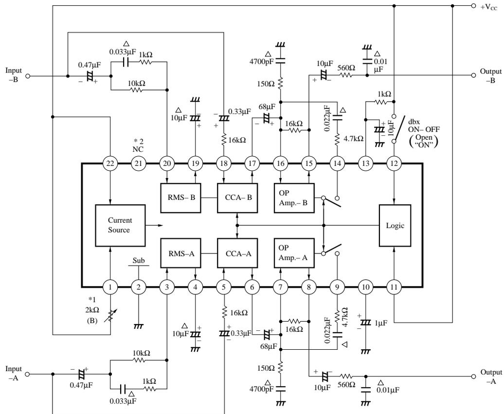
\* 1 Signals of 1kHz, 20mV are applied to the input of the both channels, adjust sinking current into the Pin13 to  $15\mu\text{A}\pm 5\%$ . Standard value at  $V_{CC}=3\text{V}$  is about  $1\text{k}\Omega$ .
