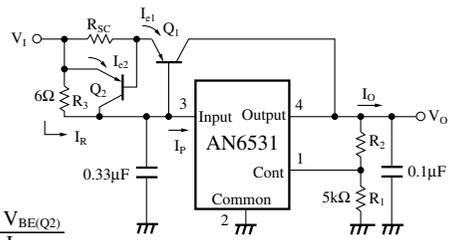
$$R_{SC} = \frac{V_{BE(Q2)}}{I_{e1(max)}}$$
