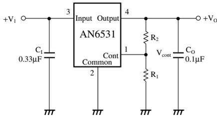
$$V_O = V_{cont} \left( \frac{R_1 + R_2}{R_1} \right)$$
