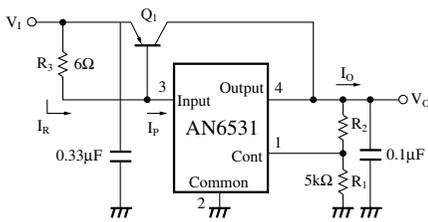
$$R_3 = \frac{V_{BE(Q1)} \cdot \beta}{(\beta + 1) I_p - I_o}$$
