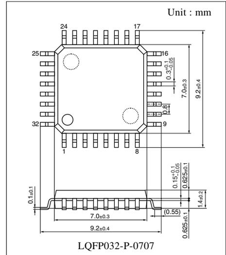
Note) The package of this product will be changed to lead-free type (LQFP032-P-0707B). See the new package dimensions section later of this datasheet.
