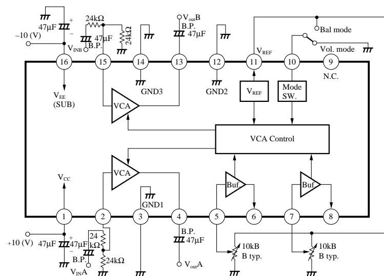
1. Voltage of Pin 7 becomes center at 1/2 V<sub>REF</sub> in case of using at balance mode.
