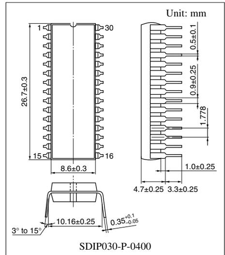
Note) The package of this product will be changed to lead-free type (SDIP030-P-0400B). See the new package dimensions section later of this datasheet.
