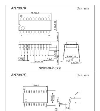
Note) The packages (SDIP020-P-0300 and SOP020-P-0300B) of this product will be changed to lead-free type (SDIP020-P-0300A and SOP020-P-0300E). See the new package dimensions section later of this datasheet.
