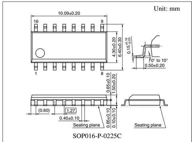
Note) The package of this product will be changed to lead-free type (SOP016-P-0225F). See the new package dimensions section later of this datasheet.
