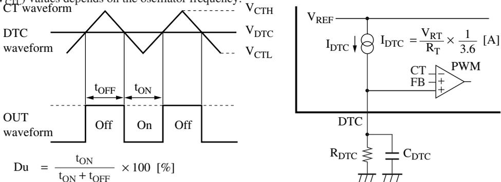
$$Du = \frac{t_{ON}}{t_{ON} + t_{OFF}} \times 100 \text{ [%]}$$
