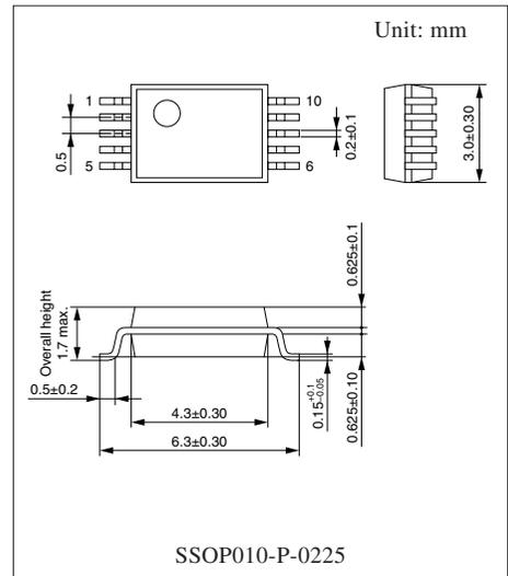
Note) The package of this product will be changed to lead-free type (SSOP010-P-0225A). See the new package dimensions section later of this datasheet.
