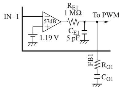
Figure 12. Error amplifier equivalent circuit (R<sub>O1</sub> inserted)
