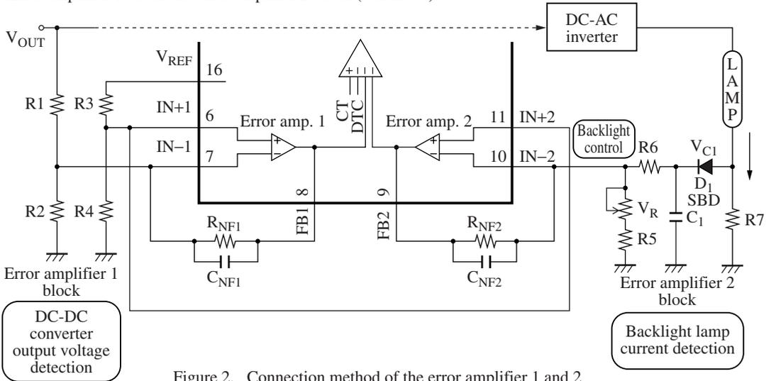
Figure 2. Connection method of the error amplifier 1 and 2
