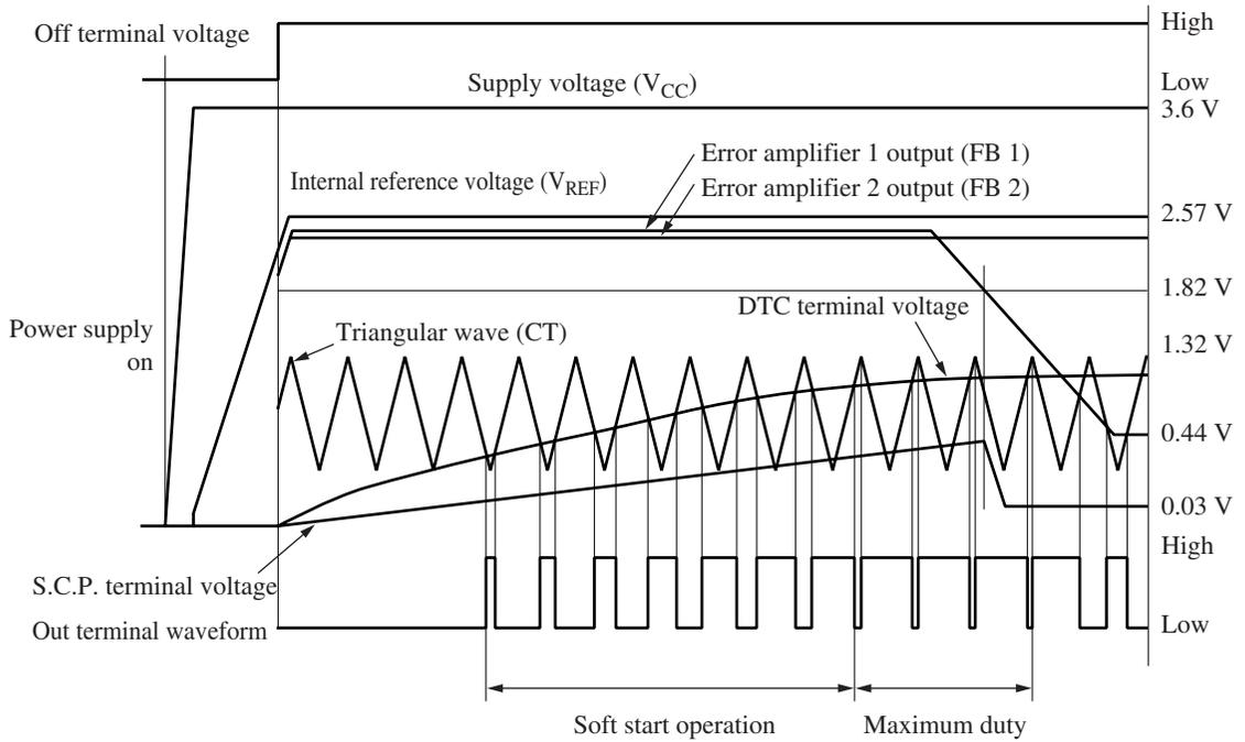
2. Short-circuit protection operation waveform
