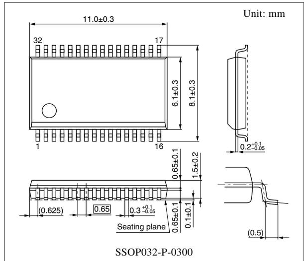
Note) The package of this product will be changed to lead-free type (SSOP032-P-0300B). See the new package dimensions section later of this datasheet.
