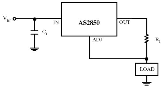
Fig. 4 5A Current output Regulator
