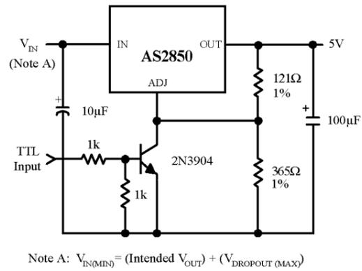
Fig.7 5V Regulator with Shutdown
