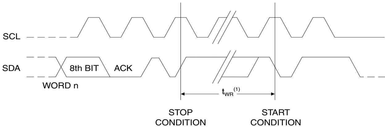
Note: 1. The write cycle time  $t_{WR}$  is the time from a valid stop condition of a write sequence to the end of the interval clear/write cycle.
