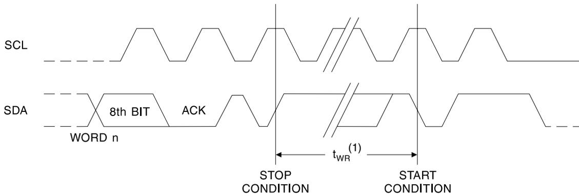
Note: 1. The write cycle time  $t_{WR}$  is the time from a valid stop condition of a write sequence to the end of the internal clear/write cycle.
