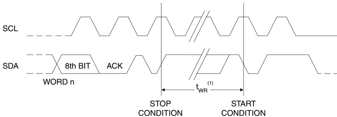
Note: The write cycle time  $t_{WR}^{(1)}$  is the time from a valid stop condition of a write sequence to the end of the internal clear/write cycle.
