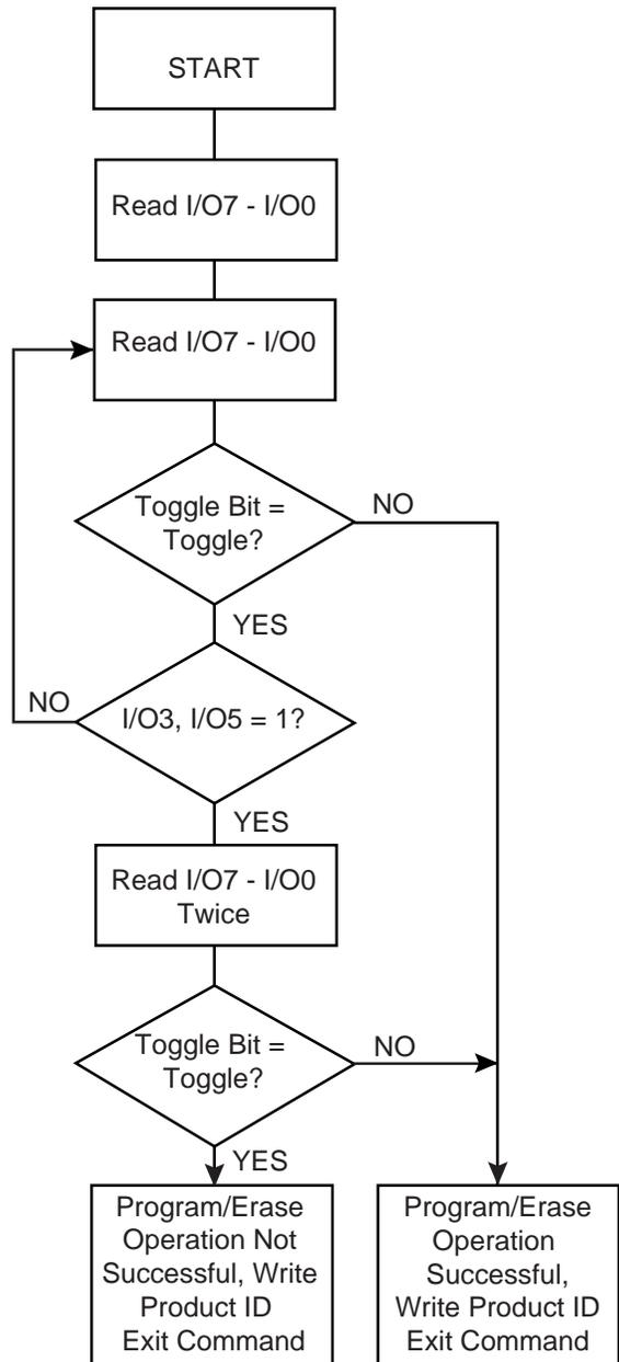
Note: 1. The system should recheck the toggle bit even if I/O5 = "1" because the toggle bit may stop toggling as I/O5 changes to "1".
