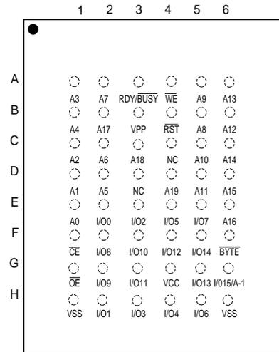
The device powers on in the read mode. Command sequences are used to place the device in other operation modes such as program and erase. The device has the capability to protect the data in any sector (see “Sector Lockdown” section).
