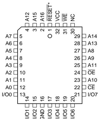
\*Note: This pin is a DC on the AT49BV001N(T) and AT49LV001N(T).
