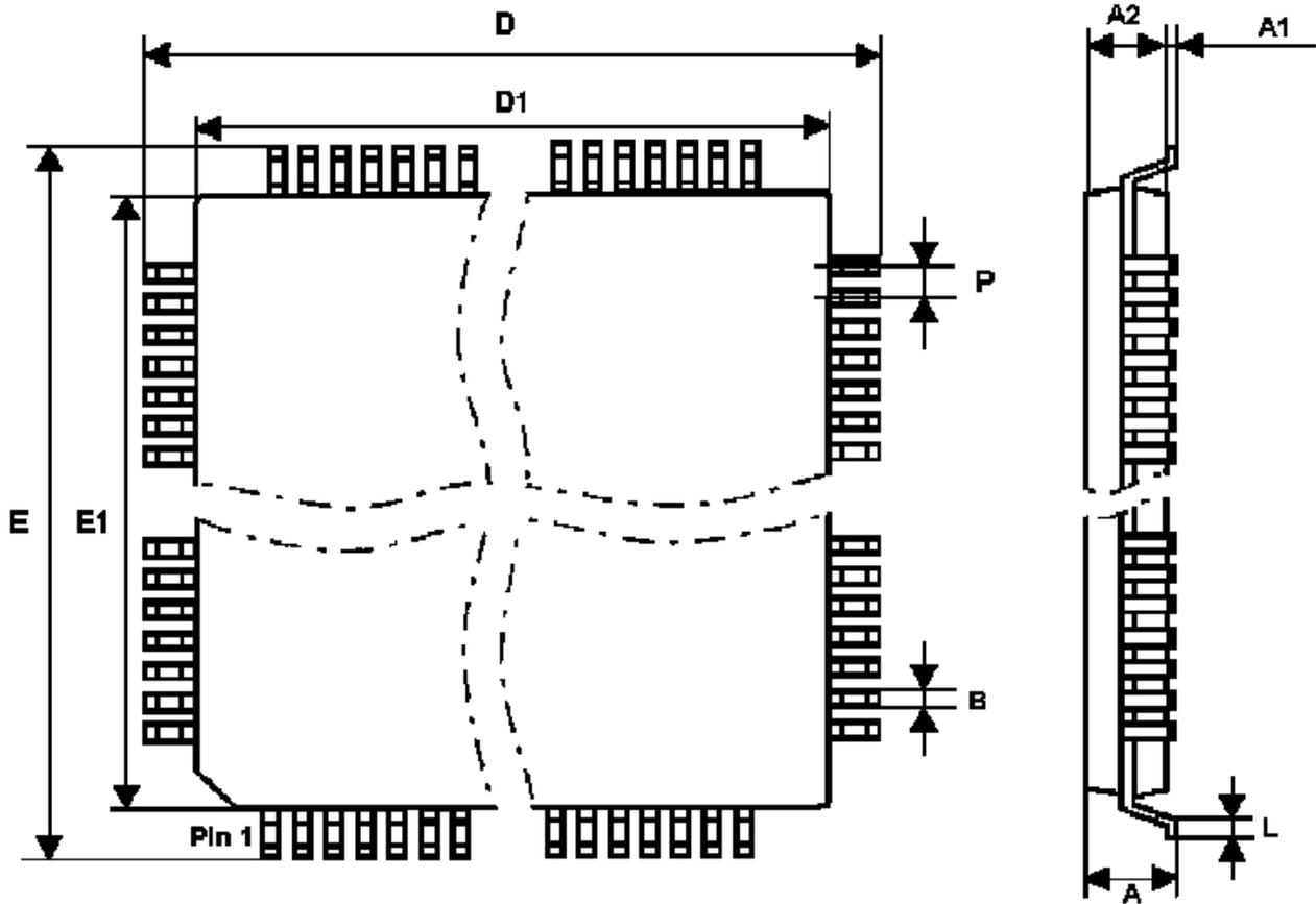
Table 19. 144-lead TQFP Package Dimensions (in millimeters)
