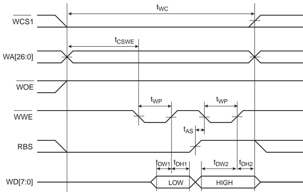
**Table 15.** External 8-bit SRAM Timing Parameters
