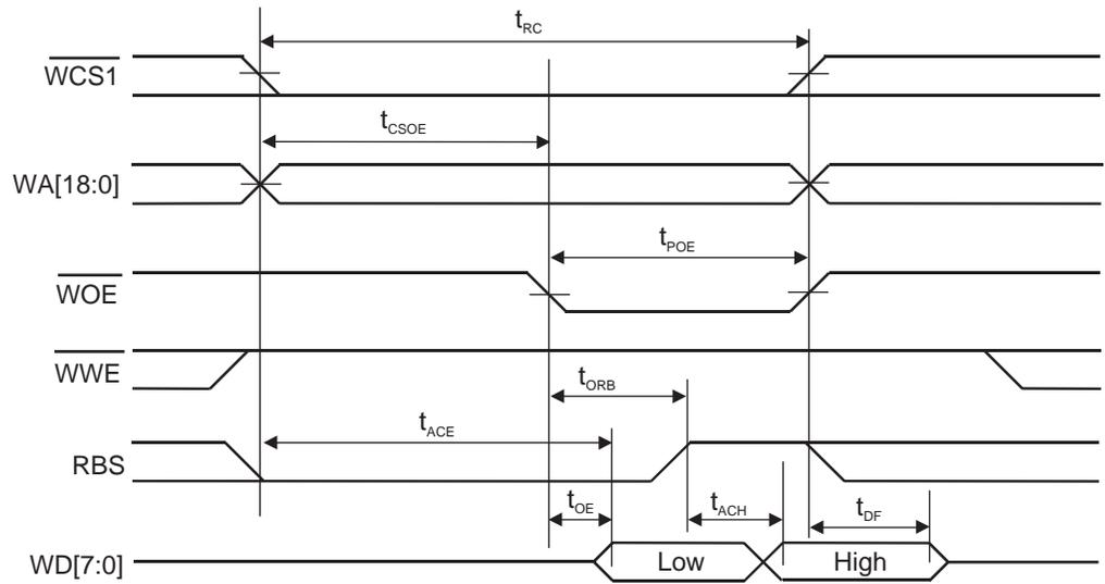
Figure 7. 8-bit SRAM Write Cycle
