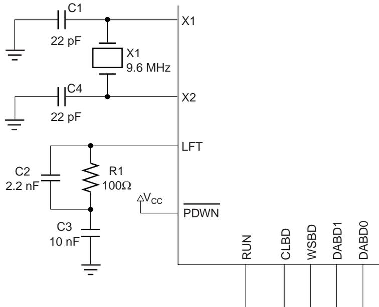
Note: The X2 output cannot be used to drive another circuit.
