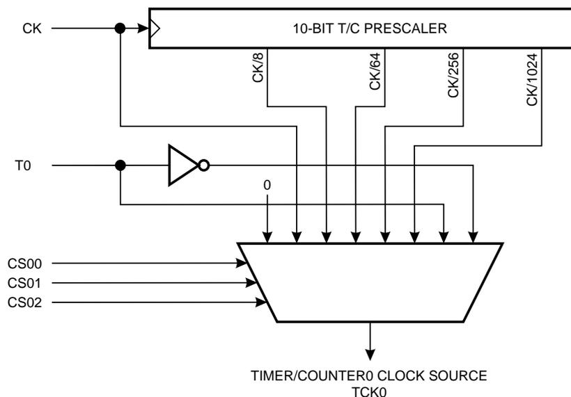
The four different prescaled selections are: CK/8, CK/64, CK/256 and CK/1024 where CK is the oscillator clock. CK, external source and stop, can also be selected as clock sources.
