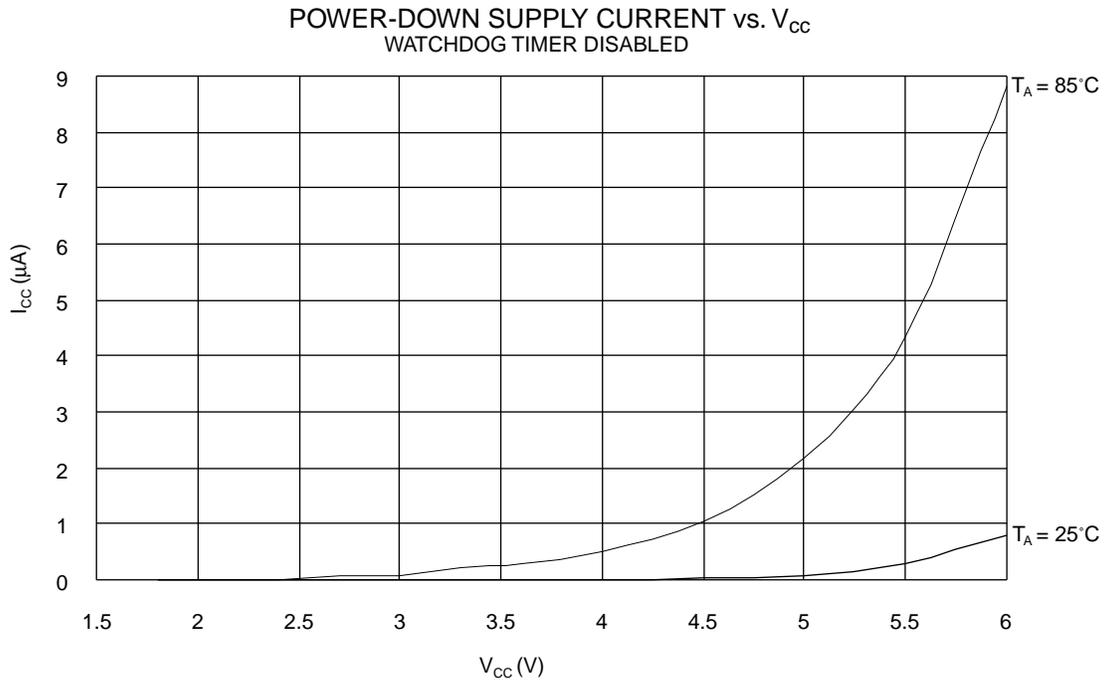
Figure 39. Power-down Supply Current vs.  $V_{CC}$
