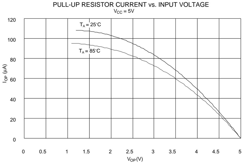
**Figure 46.** Pull-up Resistor Current vs. Input Voltage
