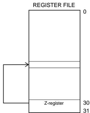
The register accessed is the one pointed to by the Z-register (R31, R30).
