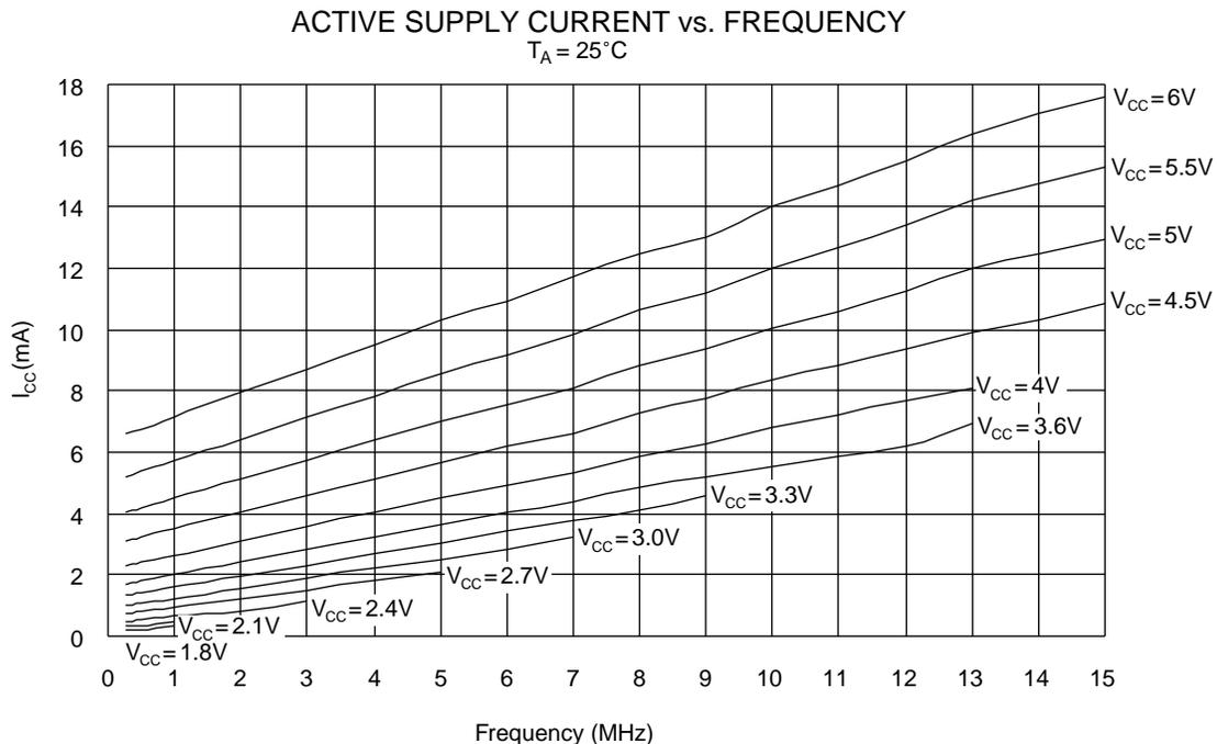
Figure 35. Active Supply Current vs.  $V_{CC}$
