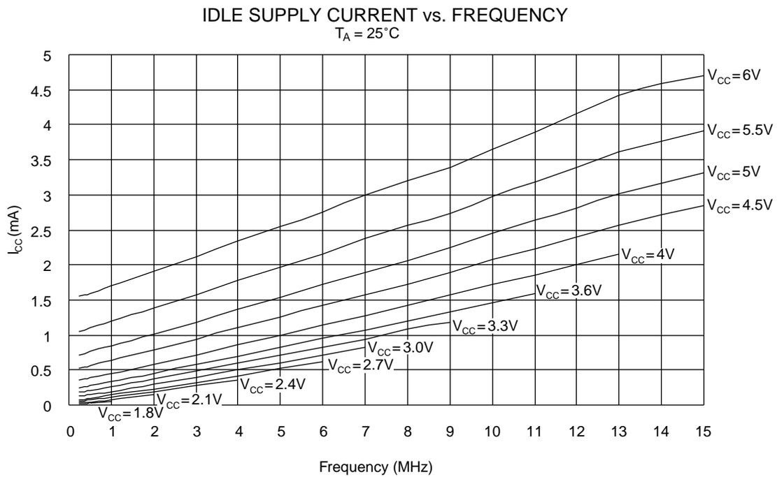
**Figure 37.** Idle Supply Current vs.  $V_{CC}$
