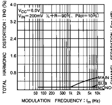
Fig. 2 Total harmonic distortion vs. modulation frequency
