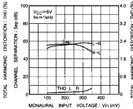
Fig. 6 Total harmonic distortion and channel separation vs. monaural input voltage
