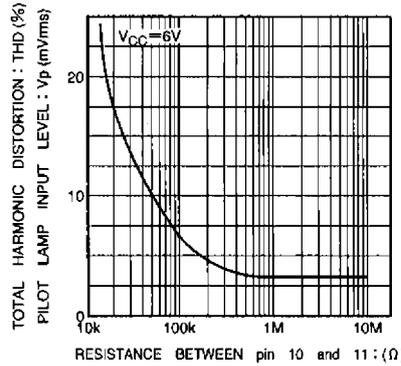
Fig. 9 Resistance between pins 10 and 11 vs. lamp on level
