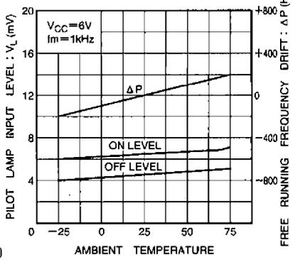
Fig. 10 Free running frequency drift and lamp on and off levels vs. ambient temperature
