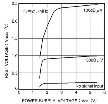
Fig. 12 RSSI voltage vs. power supply voltage
