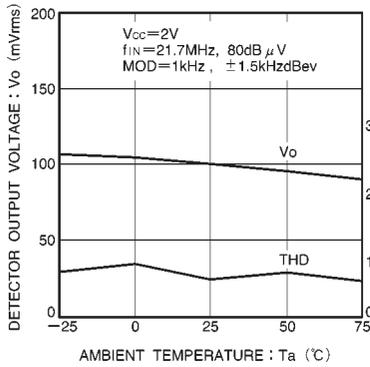
Fig. 10 Detector output level, THD vs. ambient temperature
