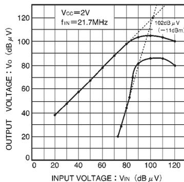
Fig. 5 Mixer output voltage vs. input voltage
