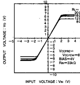
Fig. 11 Driver I/O characteristics (variable load)
