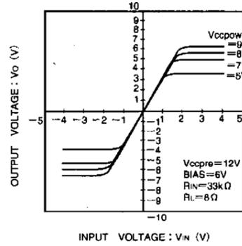
Fig. 10 Driver I/O characteristics (variable VCCPOW)
