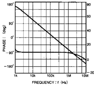
Fig. 9 Operational amplifier vs. open loop characteristics
