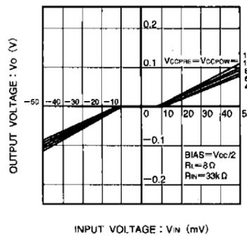
Fig. 12 Dead zone I/O characteristics
