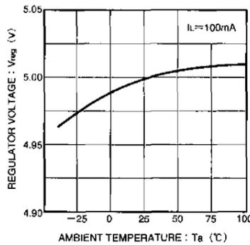
Fig. 7 Regulator voltage vs. temperature
