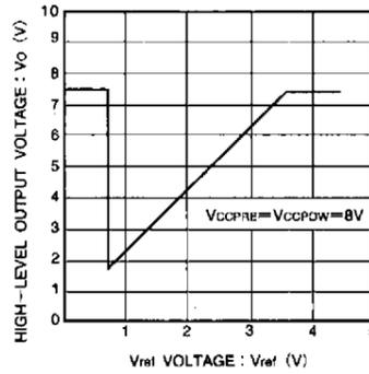
Fig. 13 Reference voltage vs. output voltage
