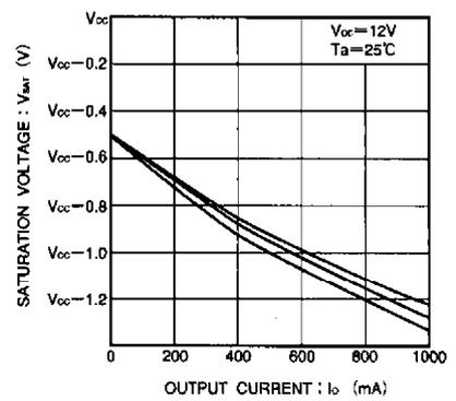
Fig.10 High-side output saturation voltage vs. output current
