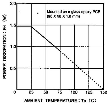
Fig.8 Power dissipation curves
