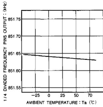
Fig. 8 1/4 frequency divider frequency vs. ambient temperature characteristics.
