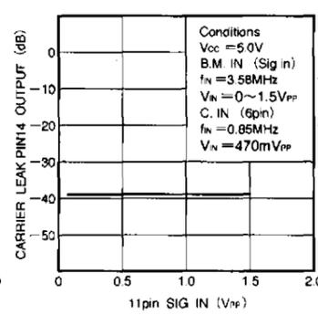
Fig. 7 B.M. carrier leak characteristics
